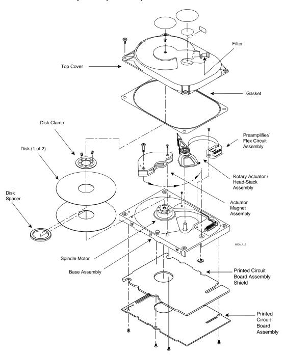
Figure 1-1 Hard Drive Components (ST31081A)
